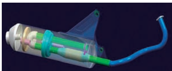
Three-part muffler to reduce exhaust noise
